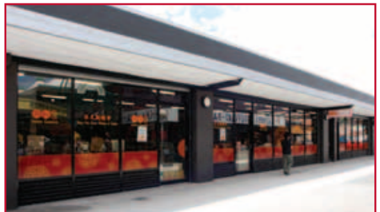
(After) A clean, fresh, bilingual logo was developed to inform the overall shopfront colour palette and signage design. The use of repeating pattern and colour on printed vinyl decals was a low-cost and visually effective method to unify the wide shopfront.
